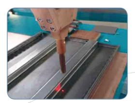
In the attached picture, it is possible to see a welding head of a "ROOF" model, the most flexible solution for assembly and manufacturing metallic doors and cabinets of any kind, available as well in its automatic version "ROBOSIDE". www.cemsa.it
